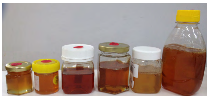
A minimum of 75 ml honey is required for the HCT. The first two jars have less than 75 ml; the next four jars have more than 75 ml. When submitting honey in a 50 ml specimen jar (second from the left), two almost-full containers are needed
