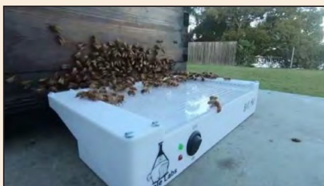
Bee venom collector - a mild electrical current on the platform the bees walk across to get to their entrance stimulates them to "sting" or release their venom. Unlike when they sting us though, they continue on unaffected. The venom is then collected from the glass plate.
